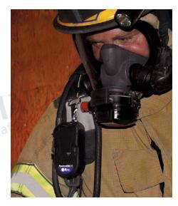
A First Responder uses the RAE Systems NeutronRAE II for audible and flashing alerts about the presence of a radiation threat and tracking of total dose exposure from gamma radiation.
