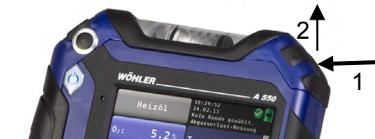
Fig. 65: Open the condensate trap compartment
