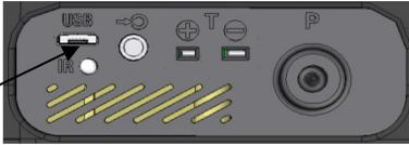
Fig. 21: USB port at the bottom
