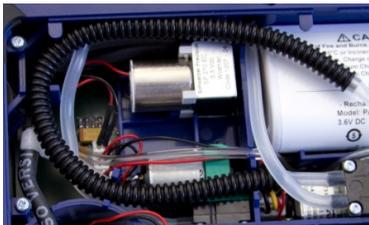
Fig. 75: Corrugated tube, correctly positioned
