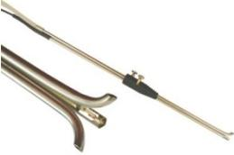
Fig. 8: S-tube probe
