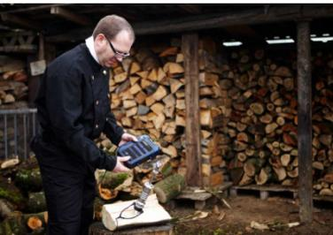
Fig. 40: Wood moisture measurement with Probe Wöhler HBF 420.
