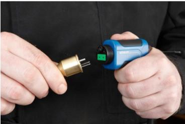
Fig. 23: Connecting the probe
