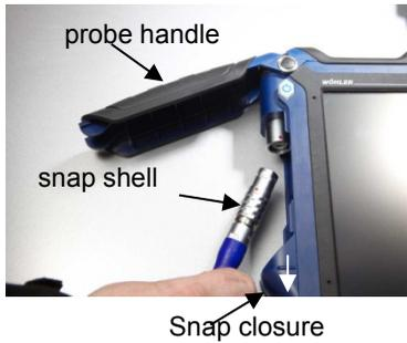
Fig. 24: Wöhler A 550 with open probe compartment
