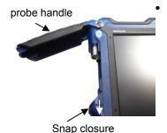
To open the probe compartment pull down the snap closure under the black probe handle.
