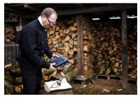
Fig. 40: Wood moisture measurement with Probe Wöhler HBF 420.
