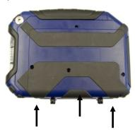
Fig. 70: Bottom of the unit - Press to open the cover.
