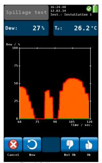
Fig. 46: Spillage test screen
