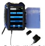
Fig. 14: Wood Moisture Probe
