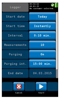
Fig. 55: Configuration of the logger measurement
