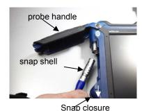
Fig. 24: Wöhler A 550 with open probe compartment
