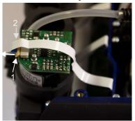
Fig. 72: Sensor with locking mechanism (1) and flexible conductor (2)
