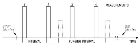
Fig. 54: schematic representation of a logger measurement
