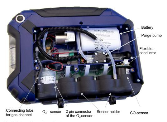
Fig. 71: Bottom of the analyzer without cover
