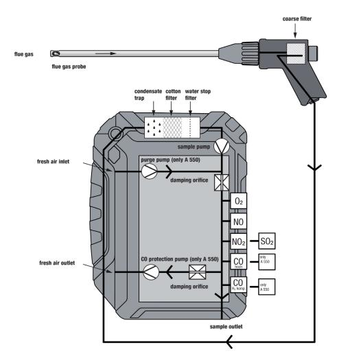
Fig. 18: Gas sampling path Wöhler A 550
