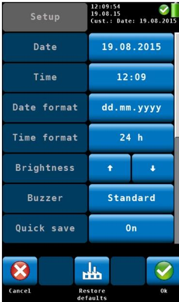
Fig. 60: Setup menu, the scroll bar shows that there are more parameters available.
