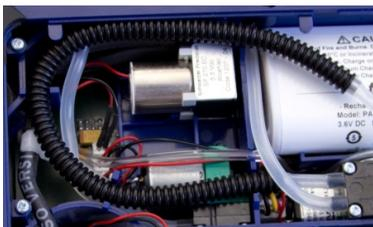
Fig. 76: Corrugated tube, correctly positioned
