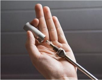
The gas probe 1,000 mm has an in-stack sinter-filter for dust protection. It removes dust ( $> 20 \mu\text{m}$ ) from the sample gas to protect the analyzer against heavy dust loads.
