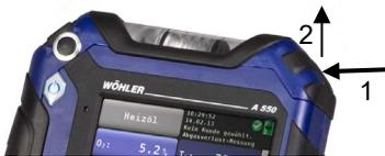
Fig. 66: Open the condensate trap compartment
