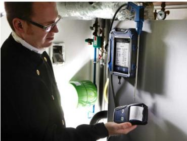
Fig. 34: Printing the readings of the Wohler A 550 INDUSTRIAL on the Thermoprinter Wohler TD 100.
