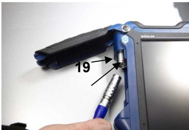
Fig. 7: Probe compartment
