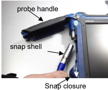
*Fig. 26: Wohler A 550 INDUSTRIAL with open probe compartment*
