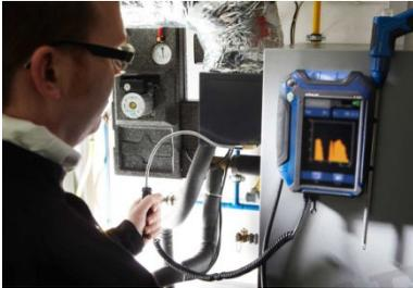
Fig. 50: Spillage test: Searching for condensate
