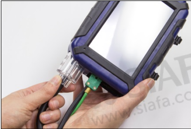
Fig. 42: Pulling the condensate trap out of the analyzer
