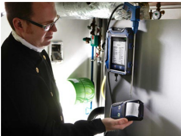
Printing the readings of the Wöhler A 450 on the Thermoprinter Wöhler TD 100.
