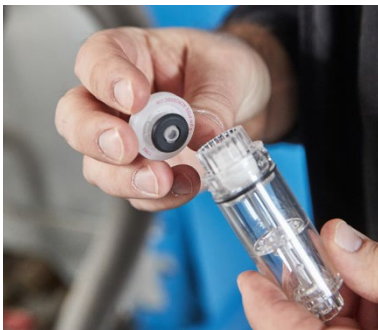
Fig. 46: Filter holder with water stop filter.
