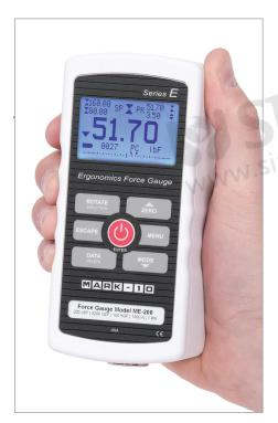
Series E push / pull force gauges make job task analysis and ergonomics analysis simple and accurate, ideal for workplace design, strength assessment, and ergonomic studies. Series E presents the ergonomist and other professionals with a simple and economical testing solution. 100 lbF, 200 lbF and 500 lbF (500, 2,500, and 5,000 N) capacity force gauges are available, along with a wide range of attachments for various applications.
