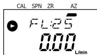
**The sensor used to measure flowrates requires time to stabilize the sensor output after the power is switched ON. Let the instrument warm up at least 10 minutes after switching the power ON. If not warmed up, it may not display correct flowrate values.**
