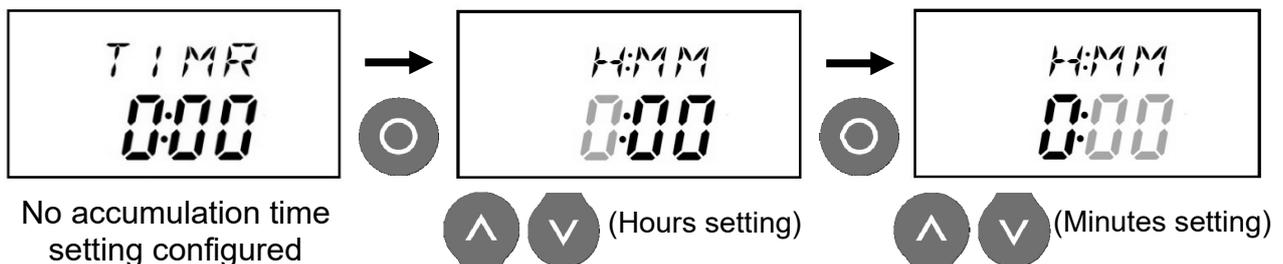
Press the [ENTER] key, which causes the hours display (hours) to flash. Then use the [UP] or [DOWN] key to set the time (hours). Once again, press the [ENTER] key, which causes the minutes display (minutes) to flash. Then use the [UP] or [DOWN] key to change the setting for minutes. Press the [ENTER] key to confirm the setting. (To return to the previous screen without changing the setting, press the [MODE/ESC] key.)
