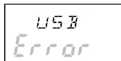
FC-L1 screen after power supply was interrupted to the low volume pump or PM2.5 sampler during automatic calibration.
