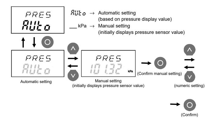
Press the [ENTER] key, which causes the display to flash, then use the [UP] or [DOWN] key to select auto or manual mode. In the manual mode, press the [ENTER] key again and then the [UP] or [DOWN] keys to change the pressure value. Press the [ENTER] key to confirm the setting. (To return to the previous screen without changing the setting, press the [MODE/ESC] key.)
