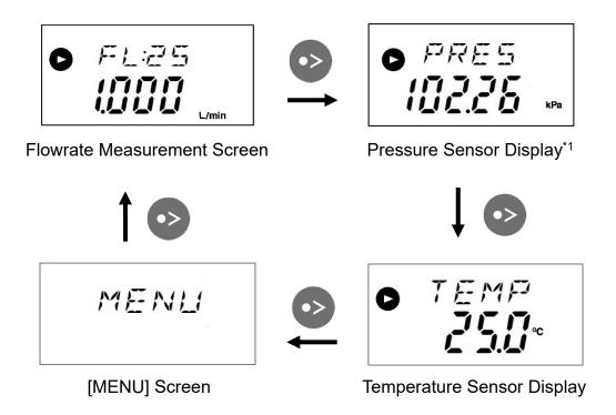
Note: It is possible to check the pressure and temperature even while measuring the accumulated and average flowrate.
