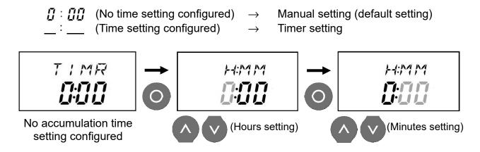
Press the [ENTER] key, which causes the hours display (hours) to flash. Then use the [UP] or [DOWN] key to set the time (hours). Once again, press the [ENTER] key, which causes the minutes display (minutes) to flash. Then use the [UP] or [DOWN] key to change the setting for minutes. Press the [ENTER] key to confirm the setting. (To return to the previous screen without changing the setting, press the [MODE/ESC] key.)
