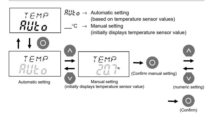
Press the [ENTER] key, which causes the display to flash, then use the [UP] or [DOWN] key to select auto or manual mode. In the manual mode, press the [ENTER] key again and then the [UP] or [DOWN] key to change the temperature value. Press the [ENTER] key to confirm the setting. (To return to the previous screen without changing the setting, press the [MODE/ESC] key.)
