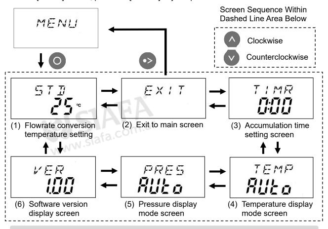
Press the [MODE/ESC] key to return to the [MENU] screen from any sub-screen in the dashed line area above.
