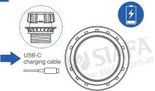
Ensure your QuantiCheck® is fully charged before use. Charging can be done via the USB-C port on the side of the device.
