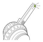
A green light illuminates on the LED indicator for a passed test.
