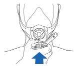
Attach QuantiCheck® to mask and don. To perform a fit check - "see point 6 on how to perform a check."
