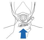
Squeeze or press and hold QuantiCheck® to perform check. Draw a breath until the blinking purple light turns solid, then hold your breath static for up to 10 seconds and wait for result.
