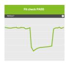
A positive pull fit check trace line shows a single large fluctuation, followed by a gently increasing line before rising again at the end of the fit check upon releasing breath.
