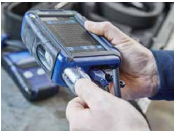
Simple maintenance – The condensate trap can easily be removed.
