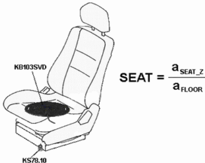
Figure 23: SEAT measurement at a drivers seat
