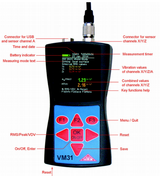
Figure 1: Controls, connectors and display
