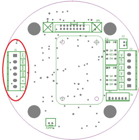
The instrument is placed in the front, on the left side of J1 terminal, the interface is 24V, GND, 4MA, GND, A (RS485A), B (RS485B) from top to bottom.
