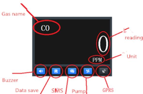
In the detection interface, the gas name is displayed in the upper left corner of the upper black area; the gas reading is displayed in the middle; the gas unit is displayed in the lower left corner. The black area below is the buzzer, data save, SMS function, air pump and GPRS status icons from left to right. The icon is blue for valid or on, otherwise the icon is gray for invalid or closed.
