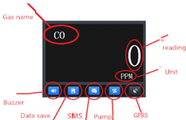
Reading: Gas concentration measured by the instrument
